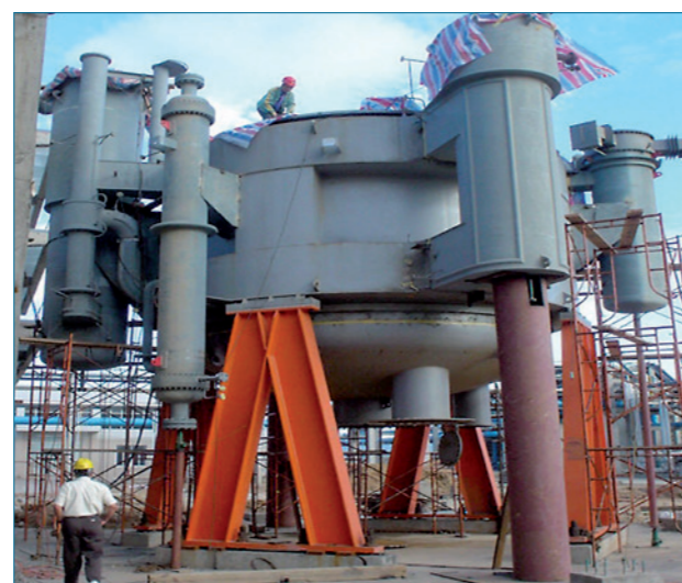
Figure 5.4: Salt-operated tubular reactors from DWE® (Source: MAN Energy Solutions).
