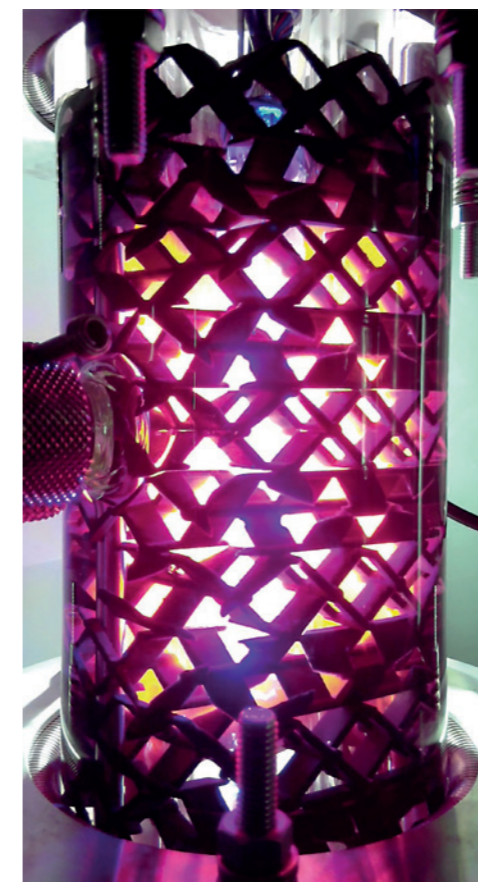
Figure 5.14: Modular miniplant photoreactor MISCOP developed by Ulm University and Peschl Ultraviolet GmbH equipped with static mixers for enhanced mass transport to improve reaction performance.
