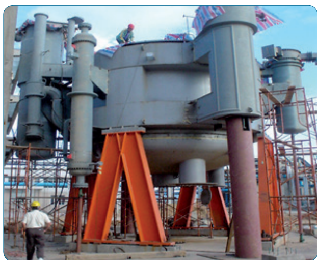
Figure 18: Salt bath reactor DWE® Reactors (source: MAN DWE GmbH).
